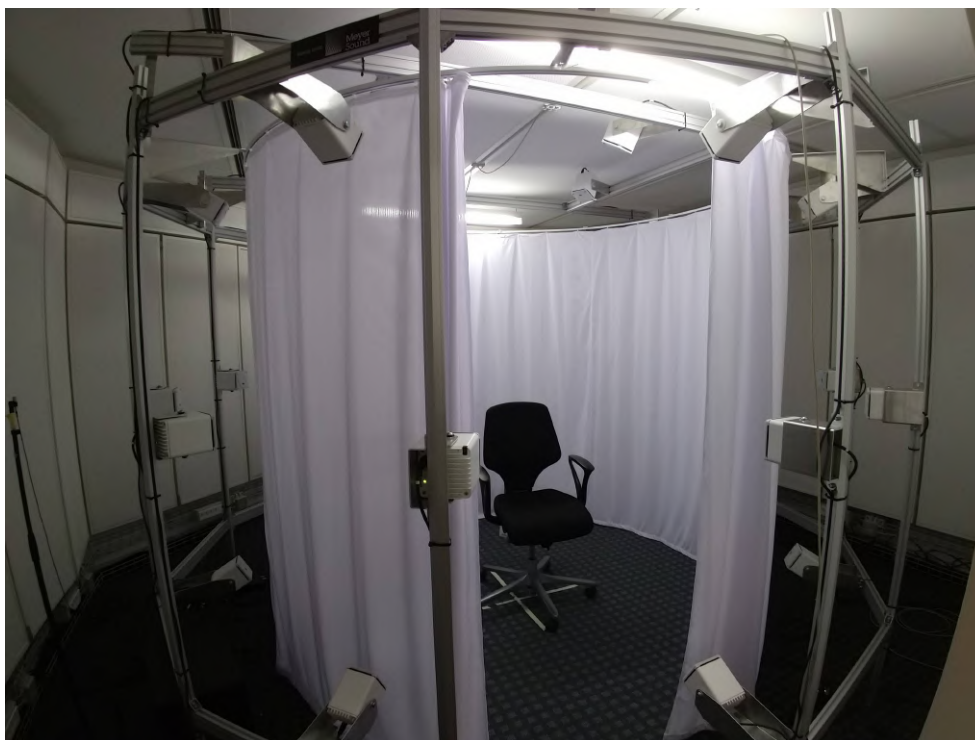
Figure 3.6 – Picture of the testing chamber. The loudspeakers are aligned spherically around the centre of the room. The curtain is acoustically transparent and shall avoid visual bias by the true loudspeaker positions or the true room dimensions. The 'X' on the floor marks the position of the sweet spot.
