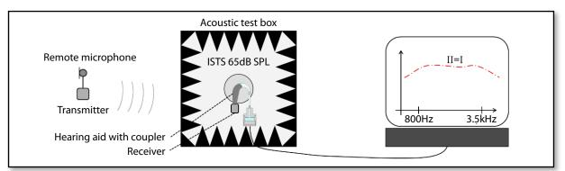
Fig. 2: Transparency measurement for hearing aids – step II – hearing aid inside the test box
