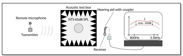
Fig. 4: Verification of the measurement conditions with empty test box
