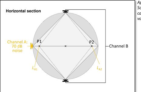
Appendix II - Fig. 3: Sound pressure levels for calculation of correction values K<sub>A1</sub> and K<sub>A2</sub>
