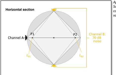
Appendix II - Fig. 4: Sound pressure levels for calculation of correction value K<sub>B</sub>
