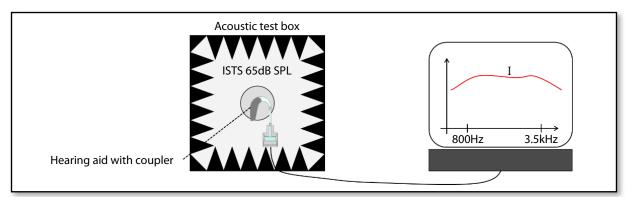
Fig. 1: Transparency measurement for hearing aids – step I - no connection to the WRM system
