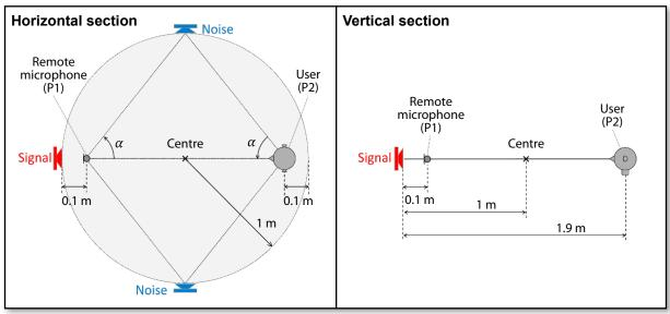
Fig. 6: Diagram of test arrangement. P1 indicates the position of the remote microphone. P2 indicates the position of the user.
