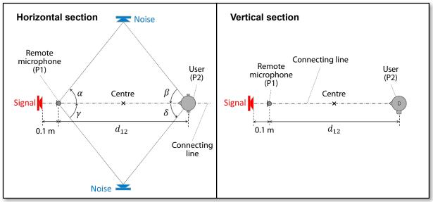
Appendix II - Fig. 5: Diagram of test arrangement in the event of deviations from the recommended geometry
