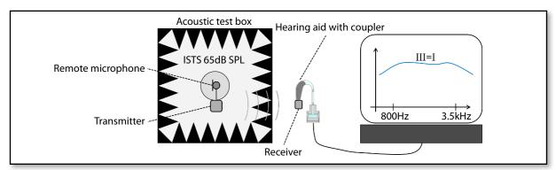
Fig. 3: Transparency measurement for hearing aids – step III – remote microphone inside the test box
