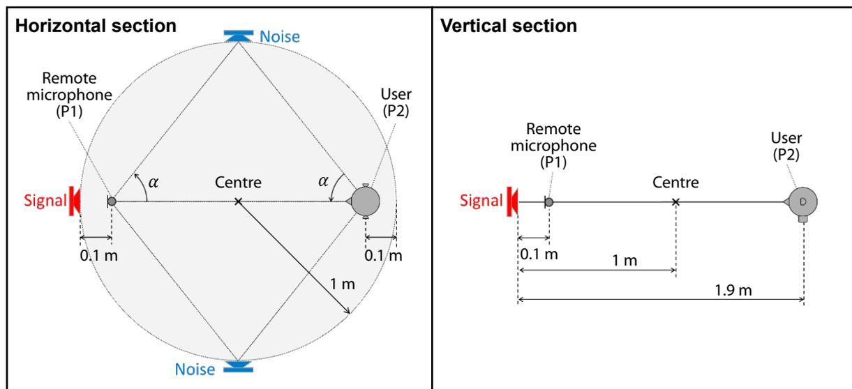
Fig. 6: Diagram of test arrangement. P1 indicates the position of the remote microphone. P2 indicates the position of the user.
