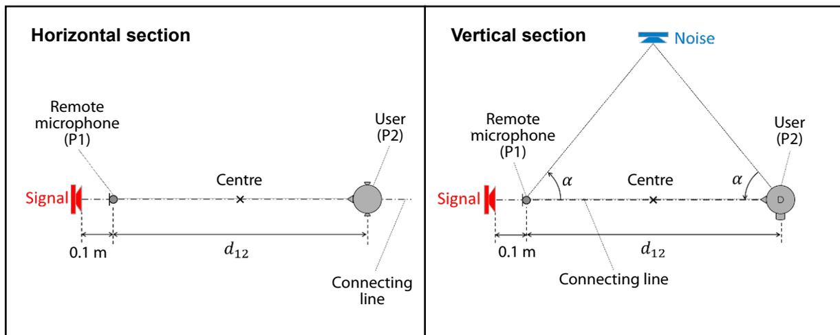
Appendix II - Fig. 6: Possible test arrangement with ceiling-mounted speaker
