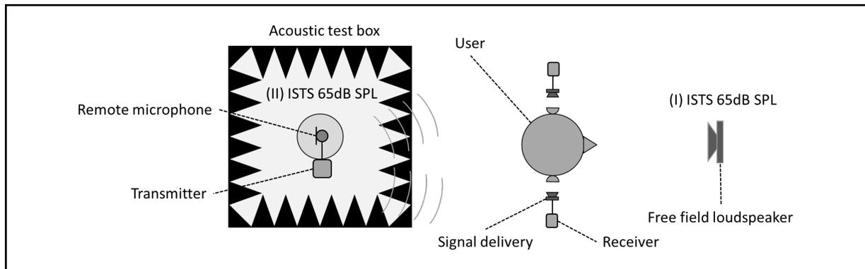
Fig. 5: Subjective evaluation of transparency. The “signal delivery” function block represents hearing aids, cochlea implants, or receiver systems for people without impaired hearing.
