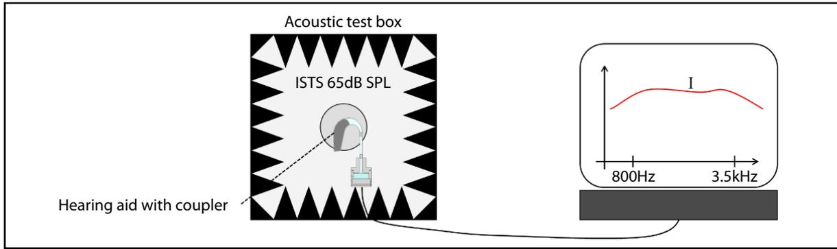
Fig. 1: Transparency measurement for hearing aids – step I - no connection to the WRM system
