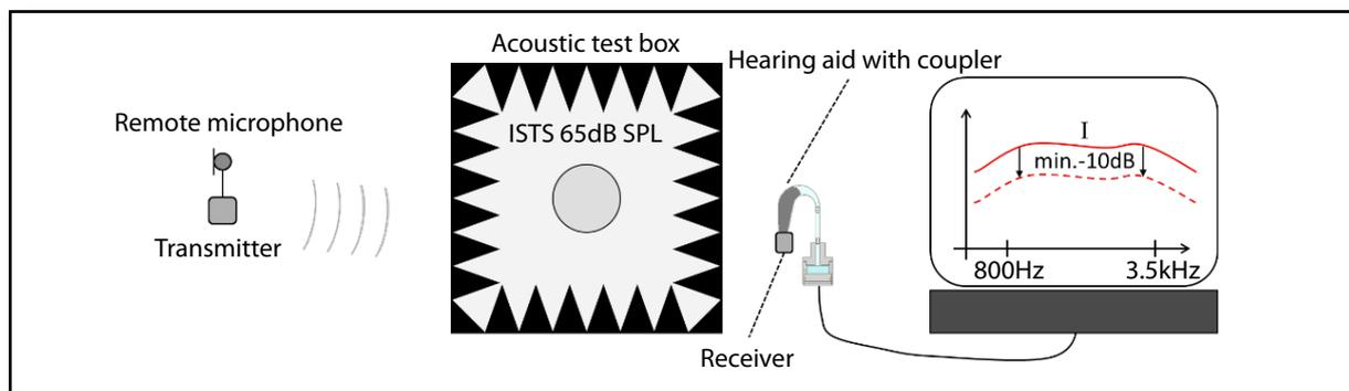
Fig. 4: Verification of the measurement conditions with empty test box
