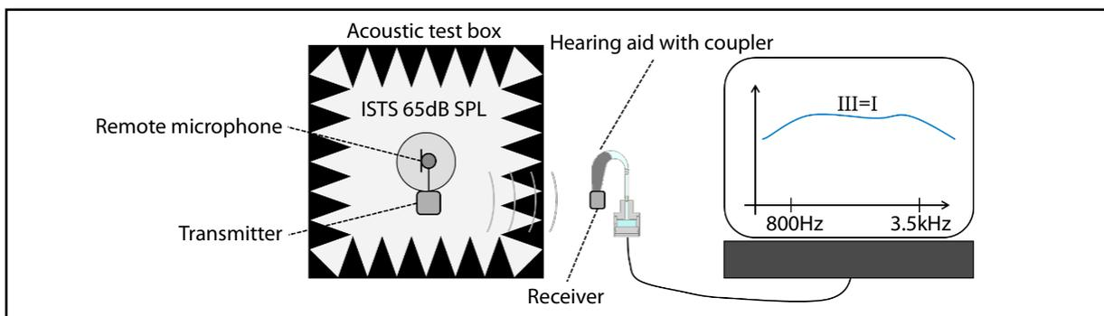
Fig. 3: Transparency measurement for hearing aids – step III – remote microphone inside the test box
