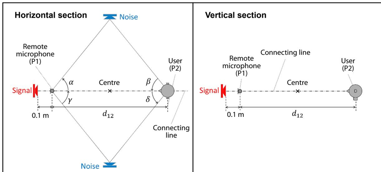
Appendix II - Fig. 5: Diagram of test arrangement in the event of deviations from the recommended geometry
