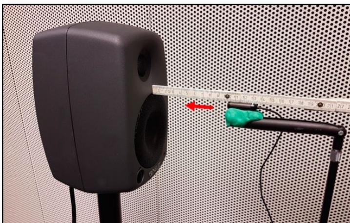
Appendix II - Fig. 2: Positioning remote microphone at a distance of 10 cm to the speaker, using a microphone stand and kneadable rubber
