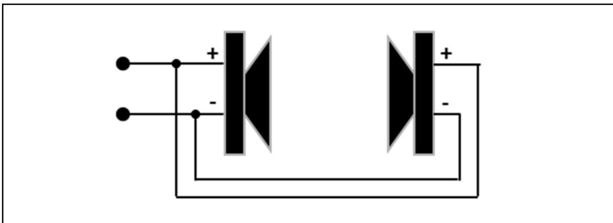
Appendix II - Fig. 1: Diagram of two speakers connected in parallel
