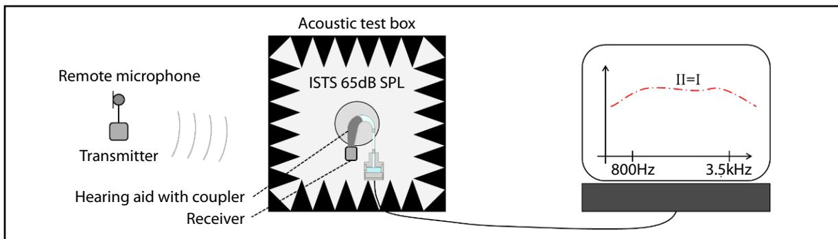
Fig. 2: Transparency measurement for hearing aids – step II – hearing aid inside the test box
