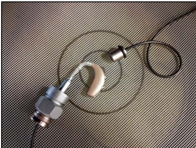
Fig. 3: Positioning of reference hearing aid and reference microphone in the test box
