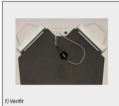
Fig. 2: Positioning of reference and measuring microphones in different test boxes
