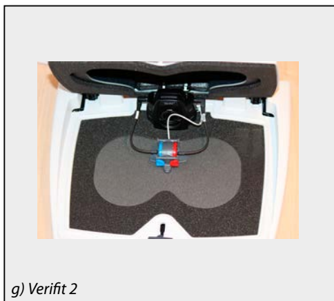
Fig. 2: Positioning of reference and measuring microphones in different test boxes
